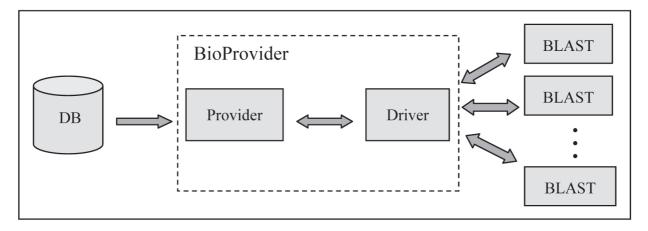
Figure 1 - The BioProvider architecture.
